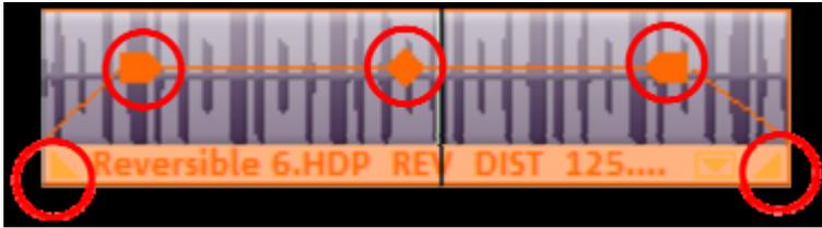
At the top corners of every object there are two fade handles that can be adjusted to fade an object (*audio, video, MIDI or text*) in or out.
